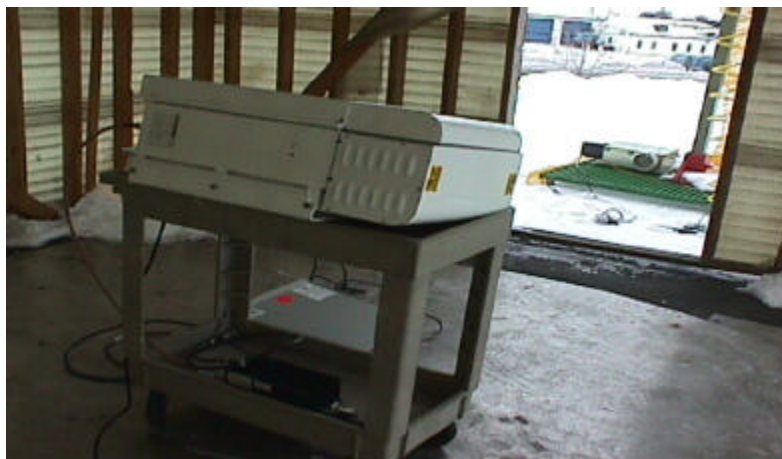
Photograph of Radiated Emissions Test Configuration
