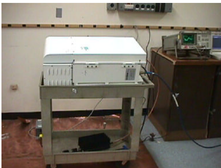
Photograph of Line Conducted Emissions Test Configuration
