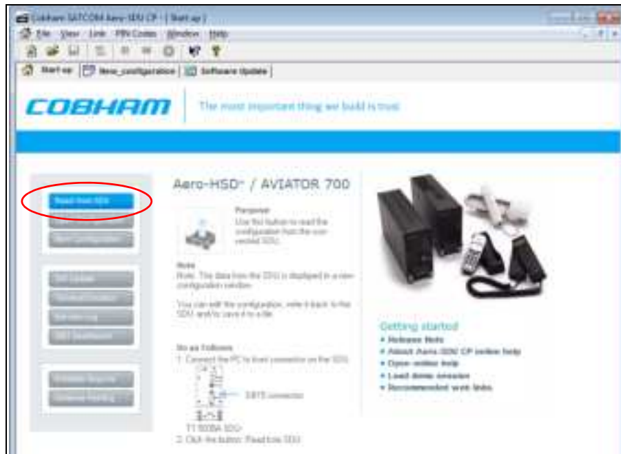
Figure C-4: Upgrading HSD+ to AVIATOR 700, SDU, step 2/7
