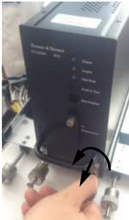
Figure 8-7: Exchanging an LRU (example)
