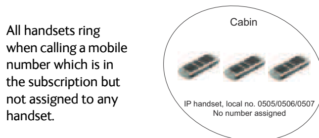
Figure 6-74: Multi-voice, example of unassigned handsets
