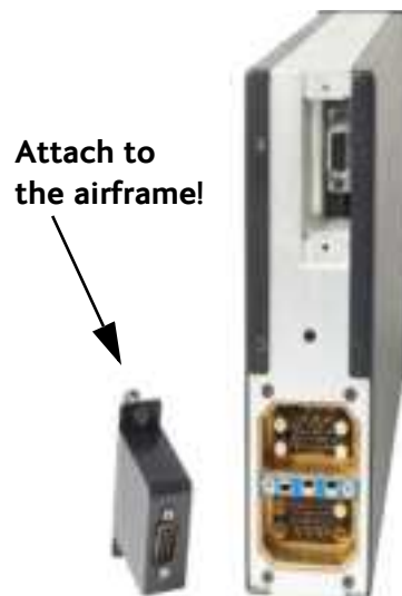
Figure 8-9: Attach CM to the airframe
