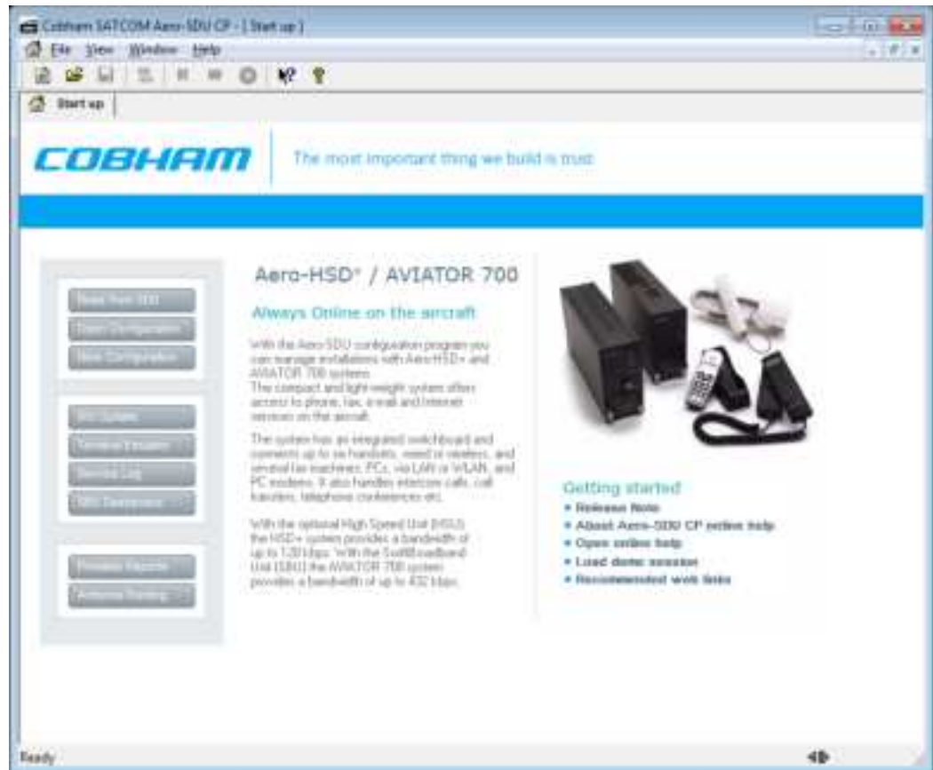
Figure 6-4: Aero-SDU Configuration Program: Start-up window
