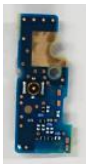
Internal Main_ANT-2-PWB (Front-side)
