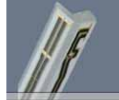
Figure 4-1 E-field Free-space Probe
