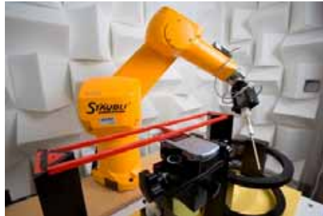
Figure 4-3 SPEAG Robotic System
