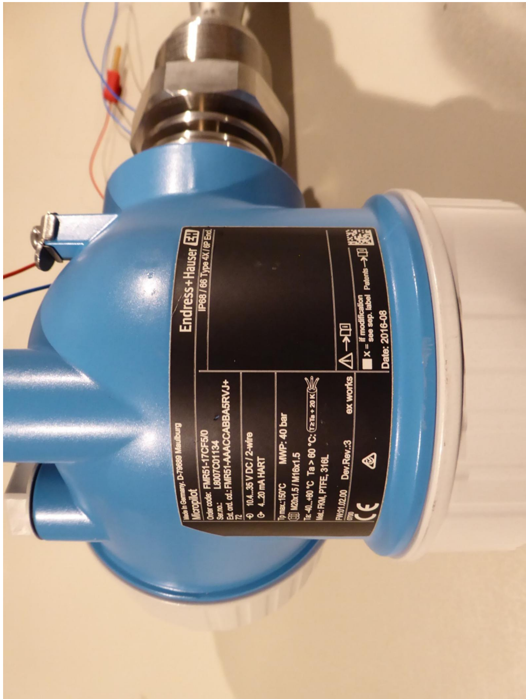
172289_c.JPG: ProToF BTLE-adaptor 2.4 GHz inside FMR51, type plate view
