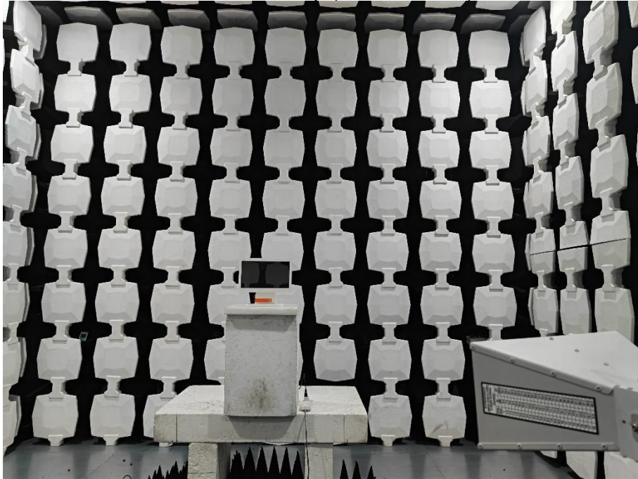
Description: Radiated Emission Test Setup (1GHz -18GHz)
