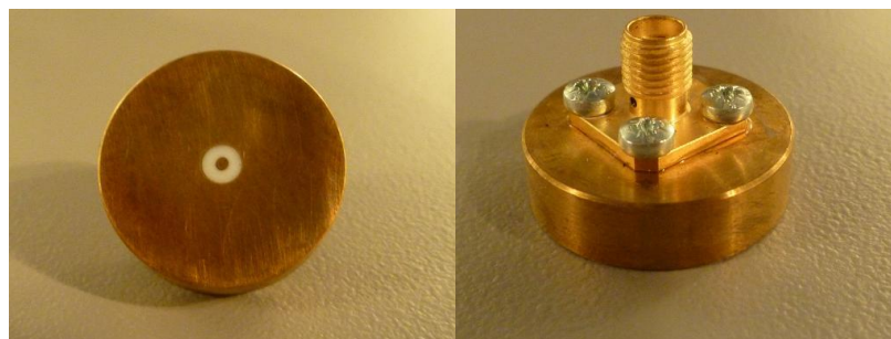
Figure 1 – MVG LIMESAR Dielectric Probe
