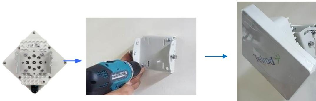
Note: The wall screws and screw anchors are not part of the package. Recommended screw size minimum 50mm length and 6-8mm diameter.
