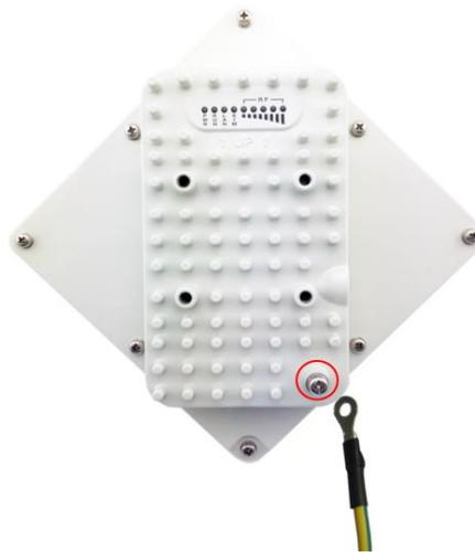
Connect one end of a grounding cable to the grounding screw and firmly tighten the grounding screw. Connect the opposite end of the grounding cable to a good ground (earth) connection.
