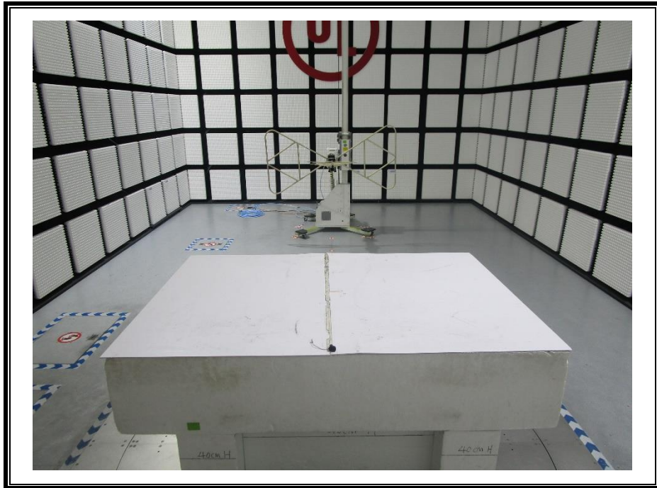
RADIATED RF MEASUREMENT SETUP (Below 30MHz)
