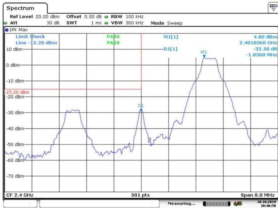
**Band Edge, Right Side**
