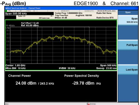
$PAPR (dB) = P_{Pk} (dBm) - P_{Avg} (dBm) = 27.46 dBm - 24.08 dBm = 3.38 dB$
