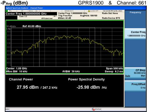
PAPR (dB) =  $P_{Pk}$  (dBm) -  $P_{Avg}$  (dBm) = 28.33 dBm - 27.95 dBm = 0.38 dB
