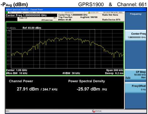
$PAPR (dB) = P_{Pk} (dBm) - P_{Avg} (dBm) = 28.35 dBm - 27.91 dBm = 0.44 dB$
