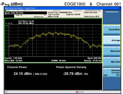
$PAPR (dB) = P_{Pk} (dBm) - P_{Avg} (dBm) = 27.55 dBm - 24.10 dBm = 3.45 dB$
