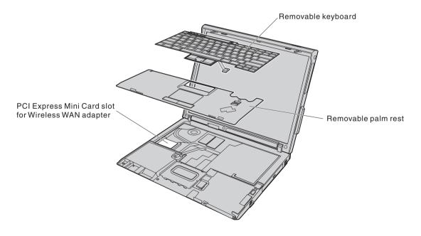
**Attention:** The ThinkPad R60 Series computer contains an authentication mechanism. If you install an unauthorized wireless WAN Mini PCI Express Card that is not approved for use in the ThinkPad R60 Series computer, the computer will not start, but only displays an error message and emits beeps.
