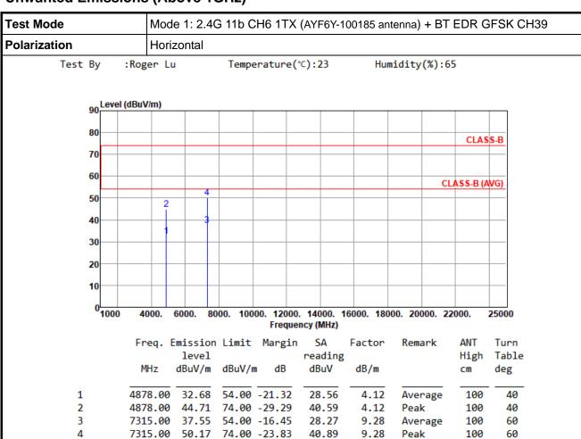
Note 1: Emission Level (dBuV/m) = SA Reading (dBuV) + Factor\* (dB/m)
