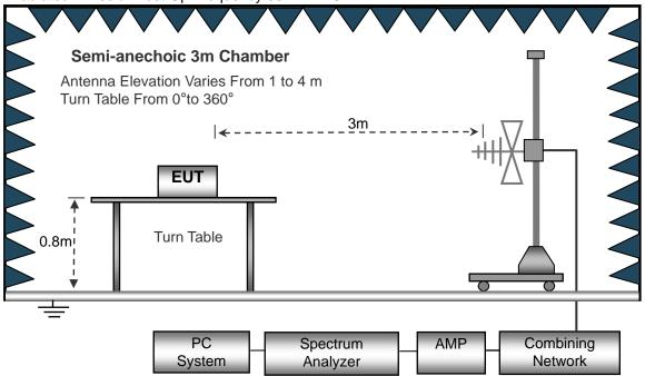
(C) Radiated Emission Test-Up Frequency Above 1GHz
