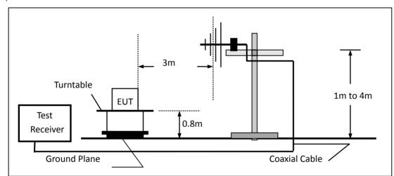
(c) For radiated emissions above 1000MHz
