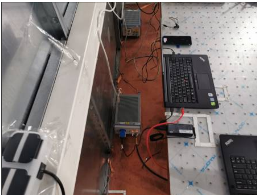
Conducted Emissions Test Setup (with laptop)
