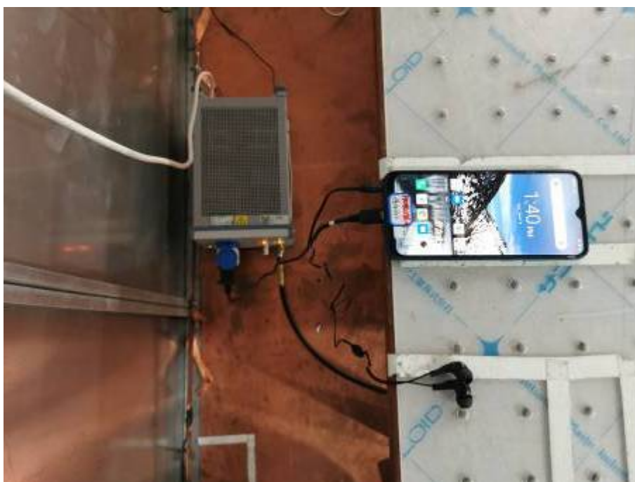
Conducted Emissions Test Setup (with charger)
