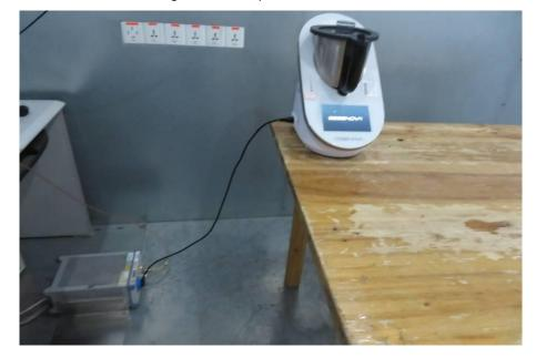
Conducted disturbance voltage at mains ports (150KHz-30MHz)
