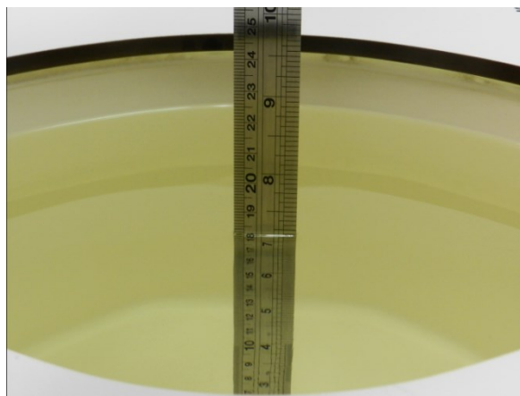
Fig 11.2 Photo of Liquid Height for Body SAR
