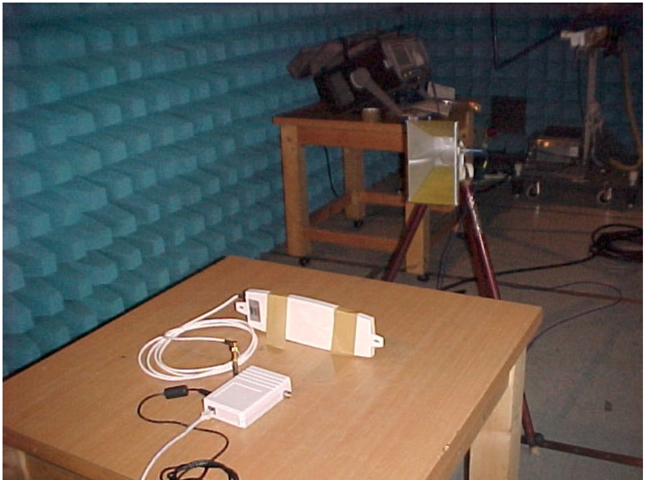
Photo #4 One Box 2.4 GHz Radio test setup
