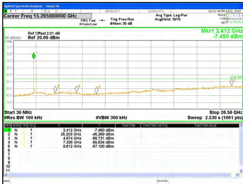
Tx. Spurious NVNT n20 2437MHz Ant1 Ref
