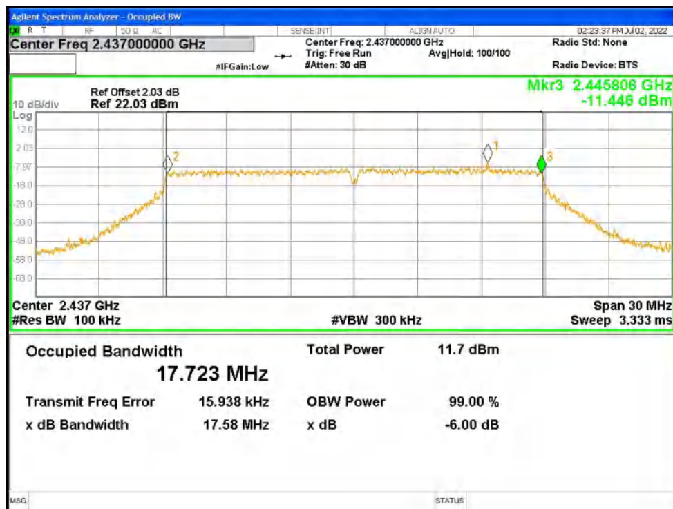
-6dB Bandwidth NVNT n20 2462MHz Ant1
