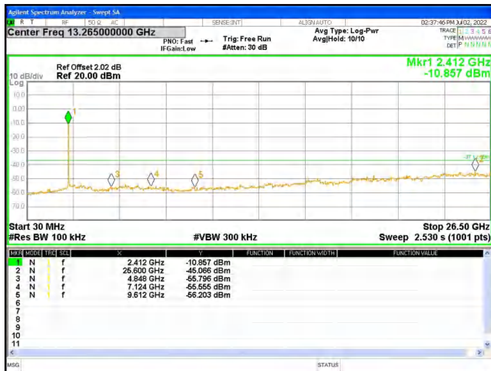
Tx. Spurious NVNT n40 2437MHz Ant1 Ref
