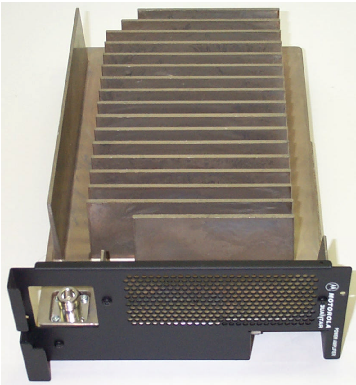
Power Amplifier Module, Heat Sink View
