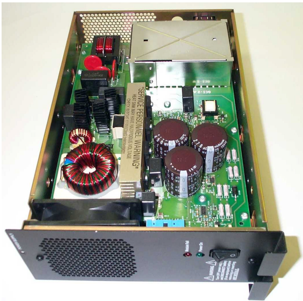
Power Supply Module, Cover Removed
