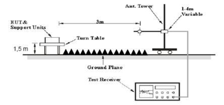
The radiated emission tests were performed in the 3 meters chamber test site for the range 30MHz to 1GHz and the 3 meters chamber B test site for above 1GHz, using the setup accordance with the ANSI C63.10-2013. The specification used was the FCC 15.209, and FCC 15.247, the RSS-247 §5.5,RSS-Gen §8.10 limits..
