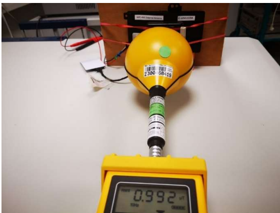
Photograph 29: Measurements in the shielded room, 9.7 cm distance between measurement probe and EUT, Position 5, H-Field, 50% charging level
