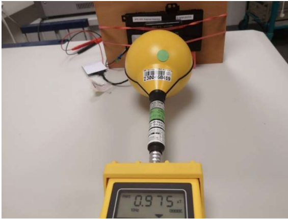
Photograph 27: Measurements in the shielded room, 9.7 cm distance between measurement probe and EUT, Position 5, H-Field, 90% charging level
