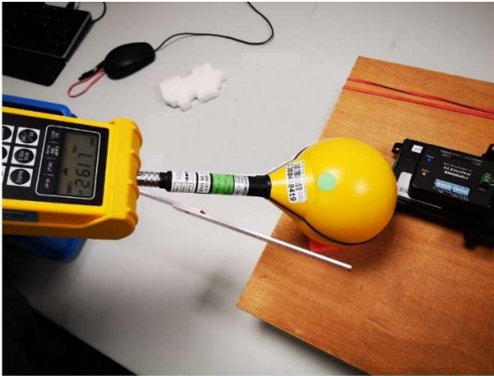
Photograph 16: Measurements in the shielded room, 6.2 cm distance between measurement probe and EUT, Position 4, H-Field, 5% charging level
