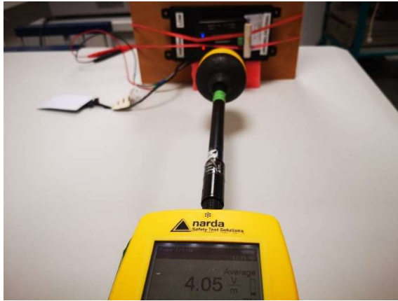
Photograph 40: Measurements in the shielded room, 9.7 cm distance between measurement probe and EUT, Position 5, E-Field, 50% charging level
