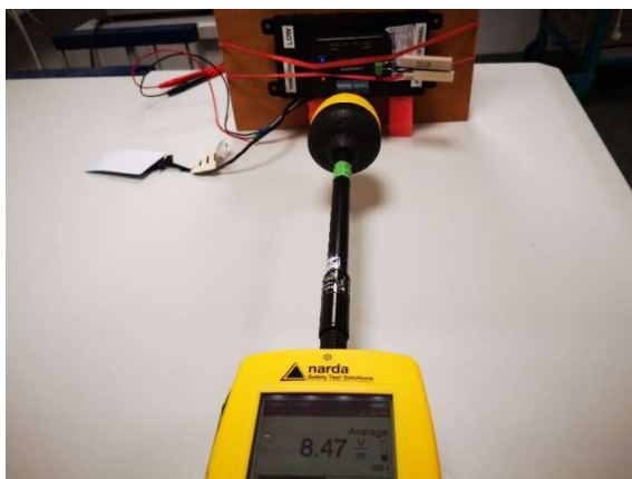
Photograph 42: Measurements in the shielded room, 9.7 cm distance between measurement probe and EUT, Position 5, E-Field, 5% charging level
