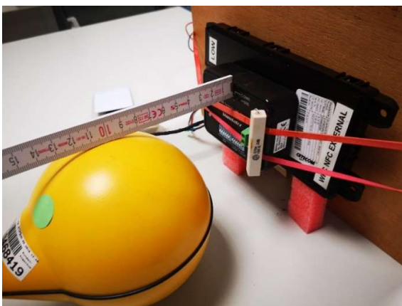
Photograph 45: Measurements in the shielded room, 9.7 cm distance between measurement probe and EUT, Position 5, H-Field, 50% charging level
