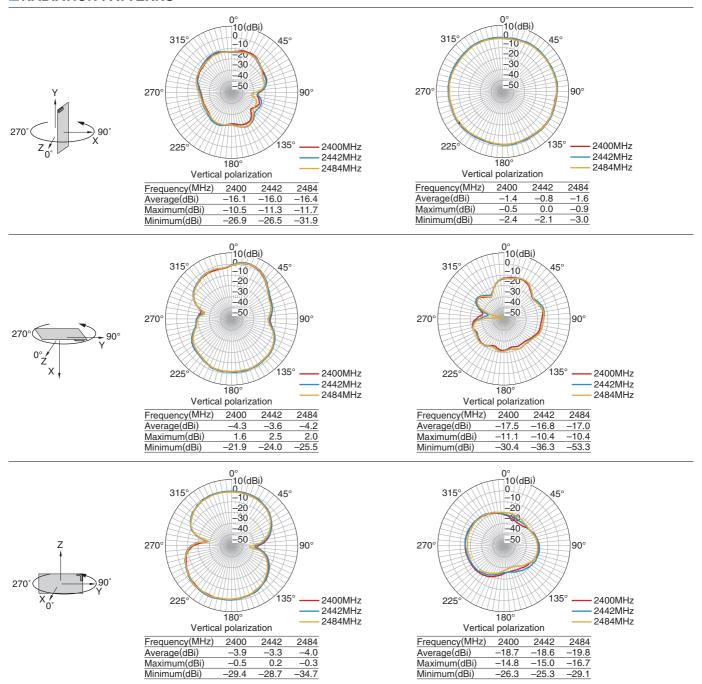
• Tested antenna has been soldered. Evaluation board size is 50x10x1 mm.
