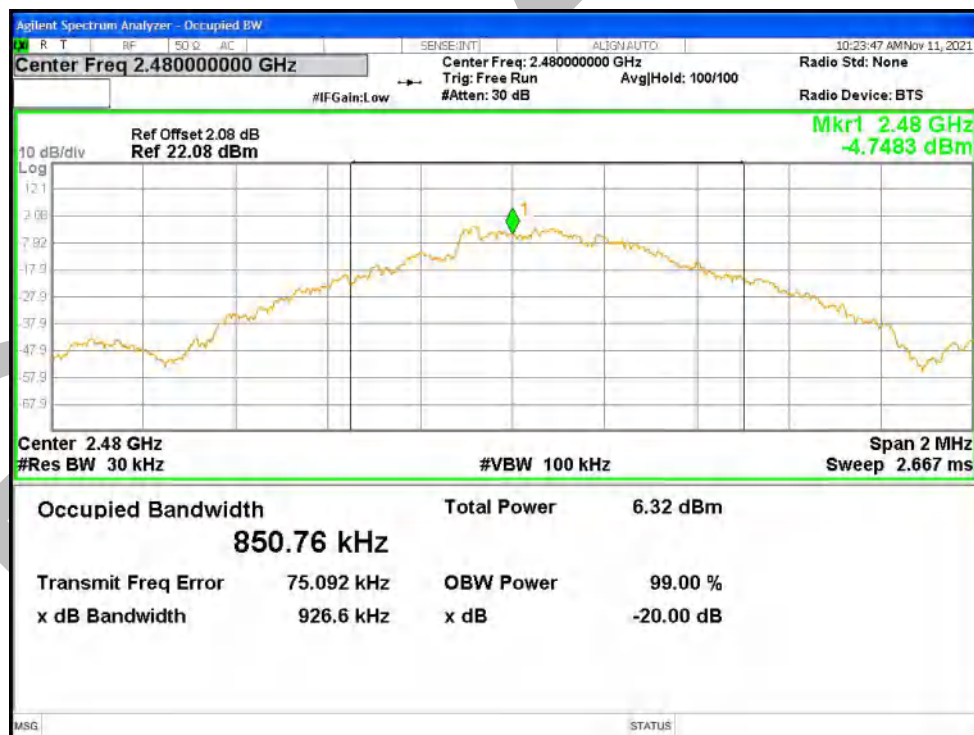
-20dB Bandwidth NVNT 2-DH1 2402MHz Ant1
