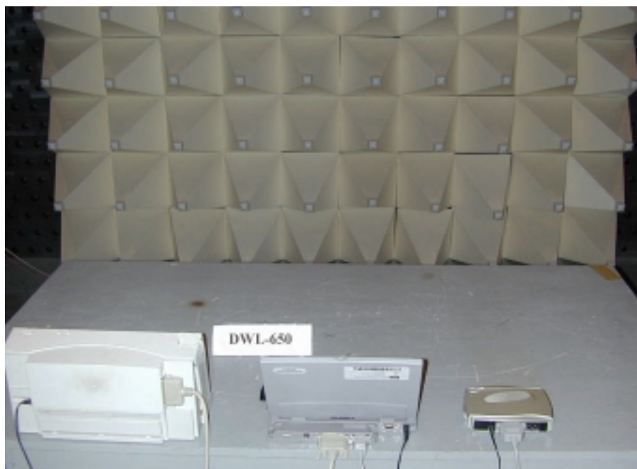
Photo 2: Spurious Test Set-up (rear)
