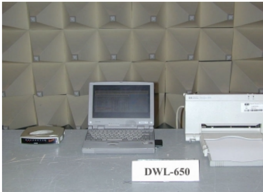
Photo 2: Spurious Test Set-up (rear)
