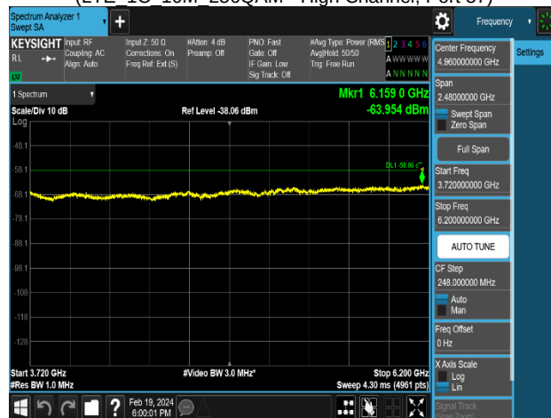
Plot 8-75. Conducted Spurious Emission Plot 3.72 GHz to 6.2 GHz (LTE_1C_20M_256QAM - High Channel, Port 57)
