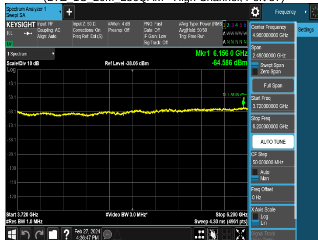
Plot 8-79. Conducted Spurious Emission Plot 3.72 GHz to 6.2 GHz (LTE 3C 20M+20M+20M QPSK - High Channel, Port 0)
