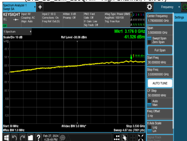
Plot 8-78. Conducted Spurious Emission Plot 30 MHz to 3.53 GHz (LTE 3C 20M+20M+20M QPSK - High Channel, Port 0)
