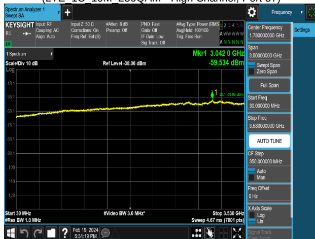
Plot 8-74. Conducted Spurious Emission Plot 30 MHz to 3.53 GHz (LTE_1C_20M_256QAM - High Channel, Port 57)
