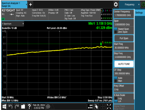
Plot 8-82. Conducted Spurious Emission Plot 30 MHz to 3.53 GHz (LTE 3C 20M+20M+20M QPSK – Non-Contiguous, Port 0)
