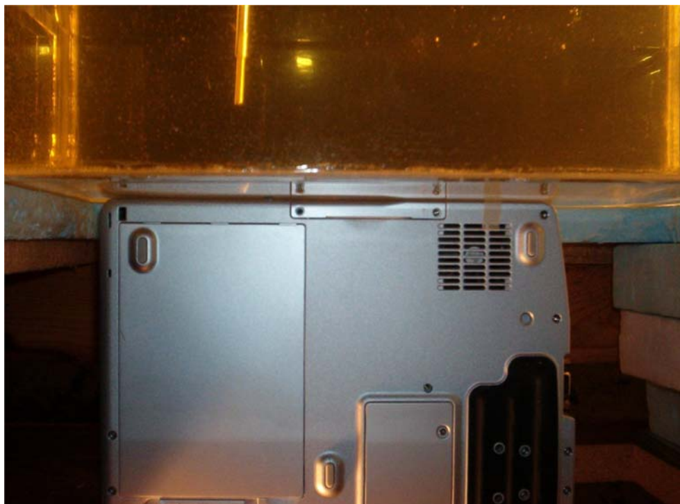
Fig. 4b. Photograph of the Gateway/Quanta Model M275DAZ/OA8 Notebook Computer with right edge of the PC at 90° pressed against the base of the planar phantom. This is Configuration 2 for SAR testing and represents the case of a bystander in contact (at a distance of 0 cm) with the right edge of the PC.
