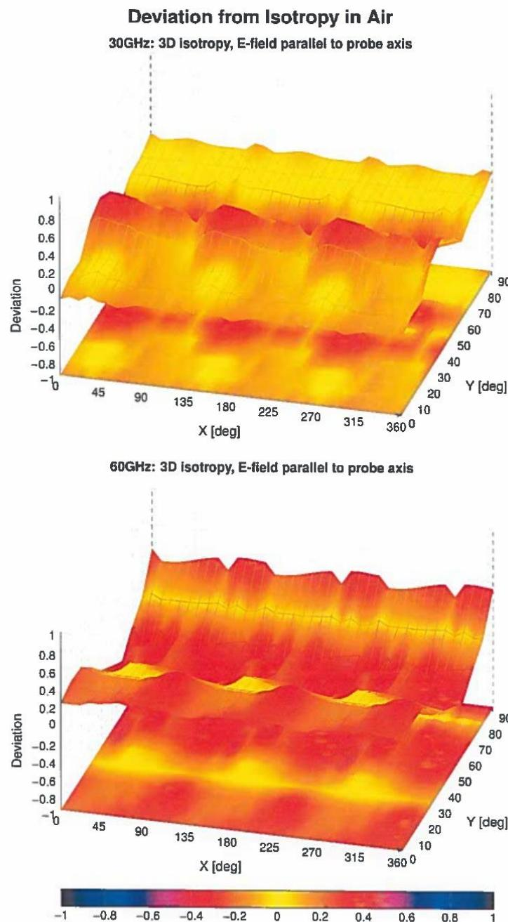
Probe isotropy for  $E_{\text{tot}}$ : probe rotated  $\phi = 0^\circ$  to  $360^\circ$ , tilted from field propagation direction  $\vec{k}$
