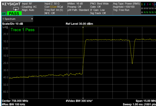
5 MHz signals, Low Band Edge, 2 carriers, nominal input signal
