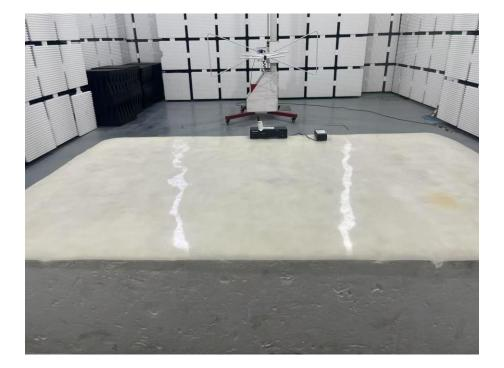
Set-up for Radiated Spurious Emission, Below 1GHz
