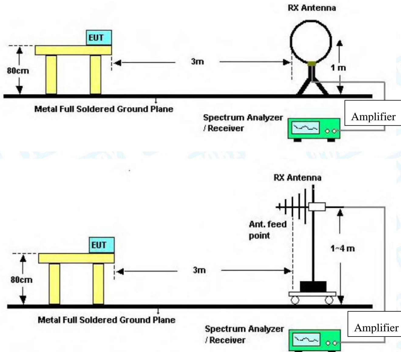
Below 30MHz Test Setup
