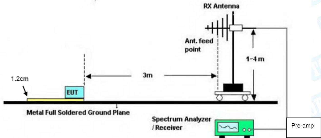
Below 1000MHz Test Setup
