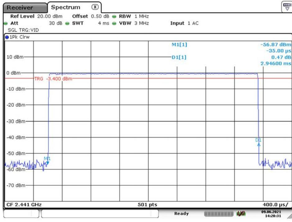
*EDR Mode ( $\pi/4$ -DQPSK):***2DH1: Middle Channel**
