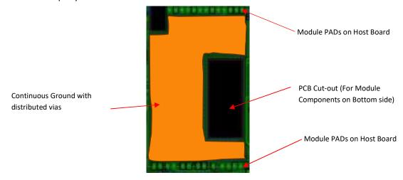
The top layer (underneath the module) of the host PCB must be ground with as many GND vias as possible.
