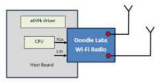
As shown in the block diagram, the modular nature of the MIMO radio module allow for accelerated development of the wireless modem. An embedded CPU with standard PCIe interface is required. Visit <u>Doodle Labs Technical Library</u> for extensive design-in documents.
