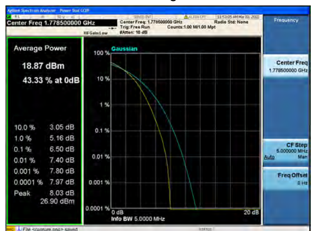
Band66 / 3MHz / High CH / 64QAM
