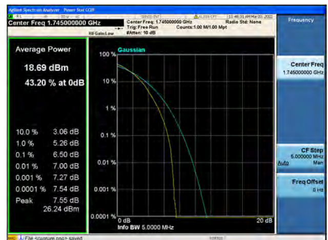
Band66 / 1.4MHz / Mid CH / 64QAM
