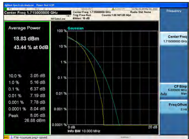
Band66 / 10MHz / Low CH / 64QAM
