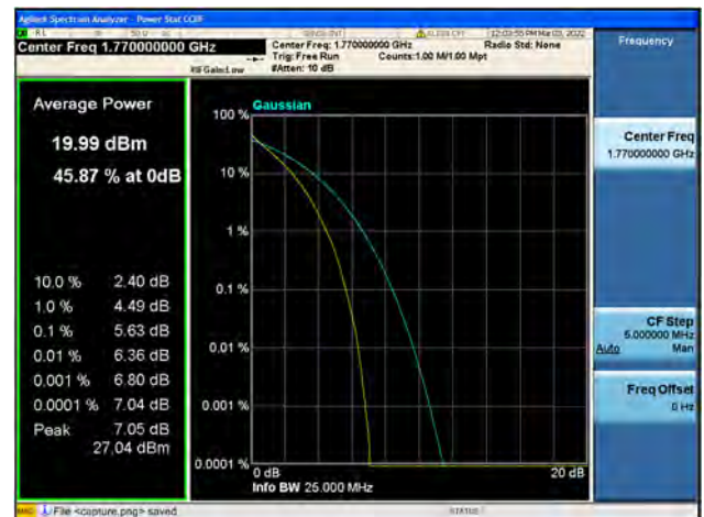
Band66 / 20MHz / High CH / 64QAM
