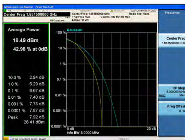
Band2 / 3MHz / Low CH / 16QAM
