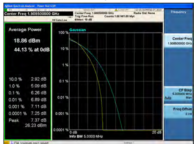
Band2 / 3MHz / High CH / 64QAM
