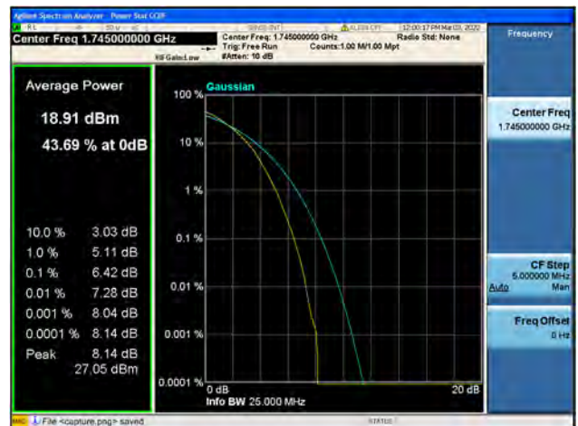
Band66 / 15MHz / Mid CH / 64QAM
