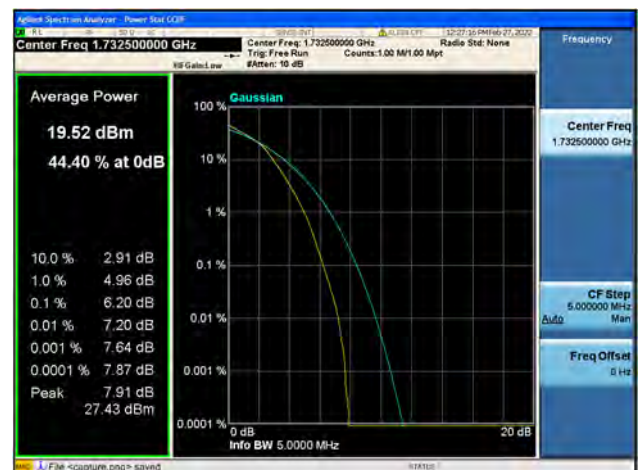
Band4 / 5MHz / Mid CH / 64QAM
