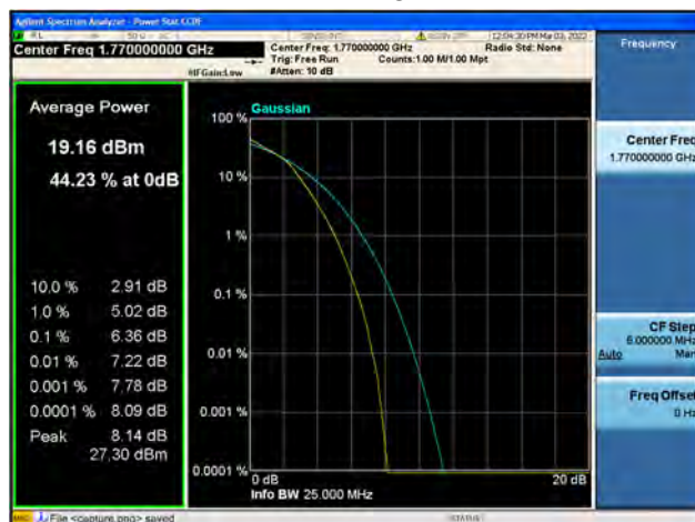
Band66 / 20MHz / High CH / 16QAM
