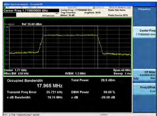
Band66 / 20MHz / High CH / 64QAM
