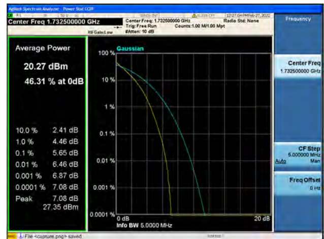
Band4 / 5MHz / Mid CH / 64QAM
