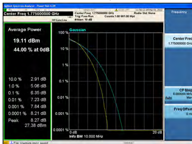
Band66 / 10MHz / High CH / 16QAM
