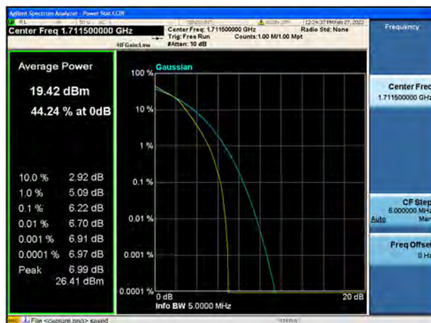
Band4 / 3MHz / Low CH / 16QAM
