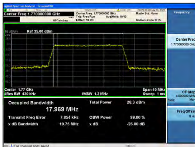
Band66 / 20MHz / High CH / 16QAM
