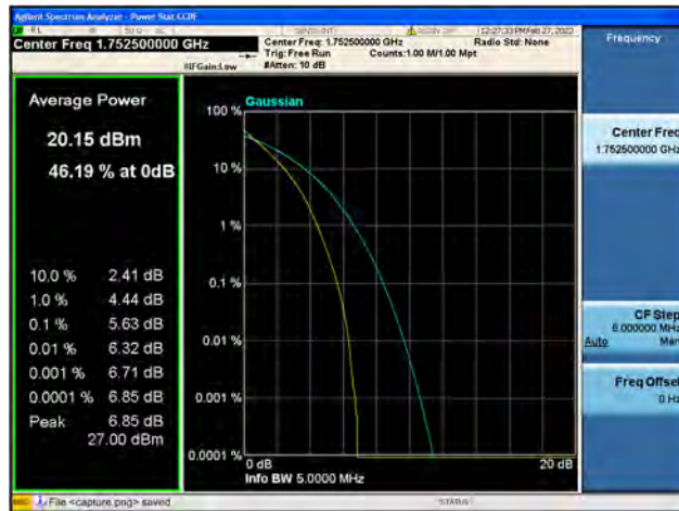
Band4 / 5MHz / High CH / 64QAM
