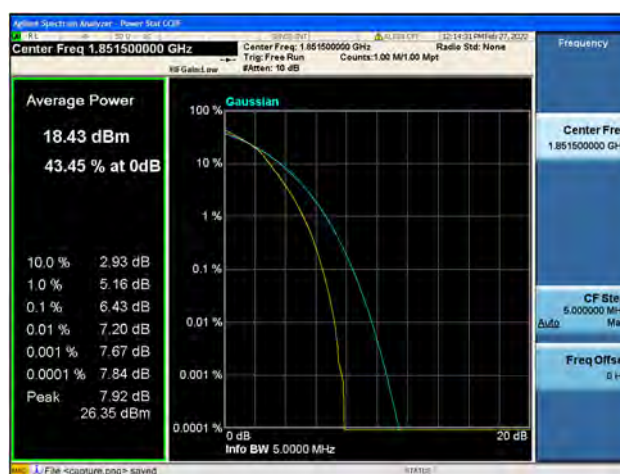
Band2 / 3MHz / Low CH / 64QAM
