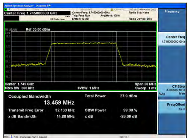
Band66 / 15MHz / Mid CH / 64QAM
