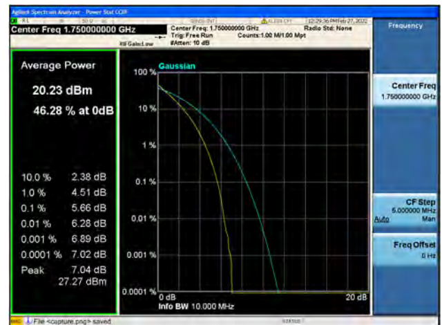
Band4 / 10MHz / High CH / 64QAM
