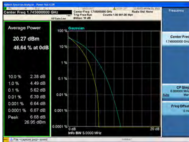
Band66 / 3MHz / Mid CH / 64QAM
