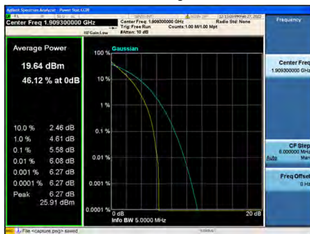
Band2 / 1.4MHz / High CH / 64QAM
