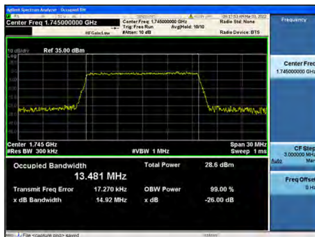
Band66 / 15MHz / Mid CH / 16QAM
