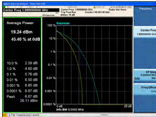
Band2 / 3MHz / Mid CH / 64QAM
