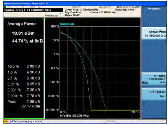
Band66 / 15MHz / Mid CH / QPSK
