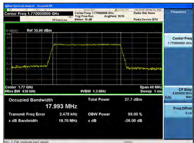
Band66 / 20MHz / High CH / 64QAM
