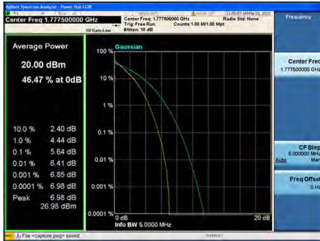
Band66 / 5MHz / High CH / 64QAM
