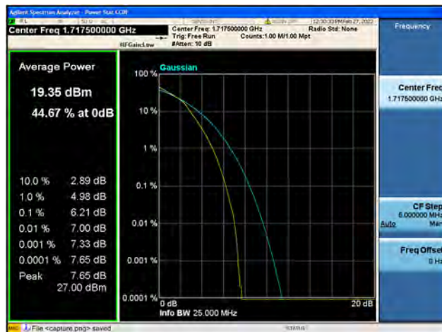
Band4 / 15MHz / Mid CH / 16QAM
