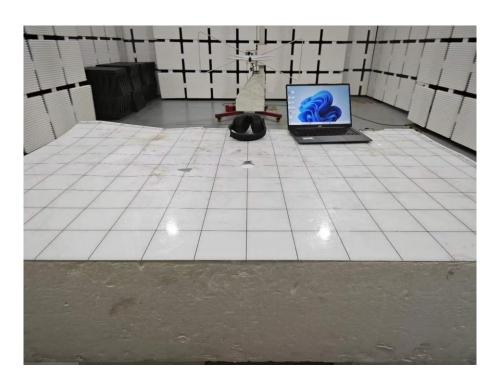
Set-up for Radiated Emission (RE), Above 1GHz
