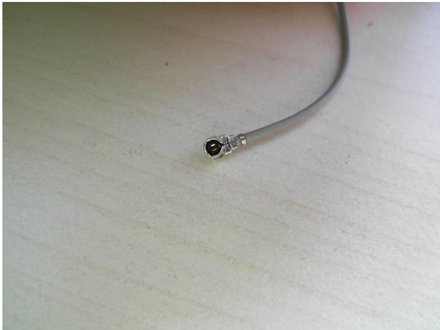
Photo 22: UFL connector at RF cable
