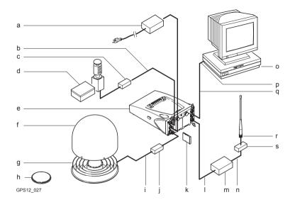
a) Power supply unit 100/240 V AC to k) CompactFlash card 12 V DC b) Interface cable Radio interface cable DB9 surge arrester with 12 V DC m) Radio pass through d) Meteo/tilt device with interface cable n) Cable to connect radio antenna Receiver GRX1200/GRX1200 Pro o) PC with, for example, Leica GPS Spider Weather protection radome for Serial port AT504 AT504 g) Data transfer cable for receiver communication h) AX1202 Radio antenna TNC to TNC antenna cable s) Radio surge arrester Surge arrester
