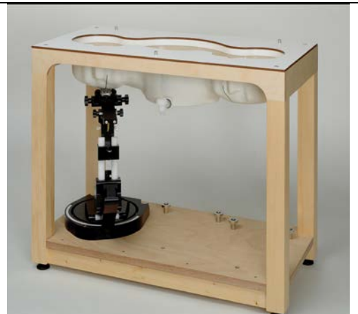
Fig. 8.7 Photo of SAM Twin Phantom
