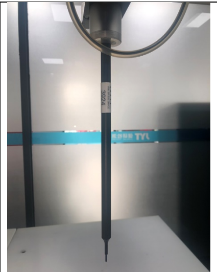
Fig. 8.2 Photo of E-Field Probe
