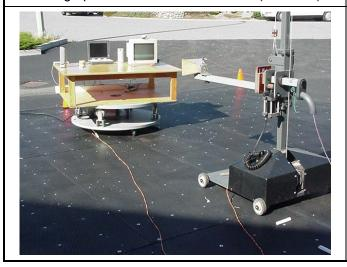
Photograph H-2 - 3160-09 Horn Antenna (18-26GHz)
