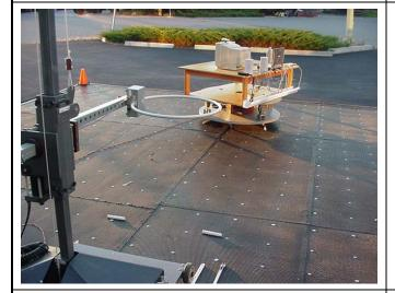
Photograph I-2 - Bilog Antenna (30MHz - 1 GHz)
