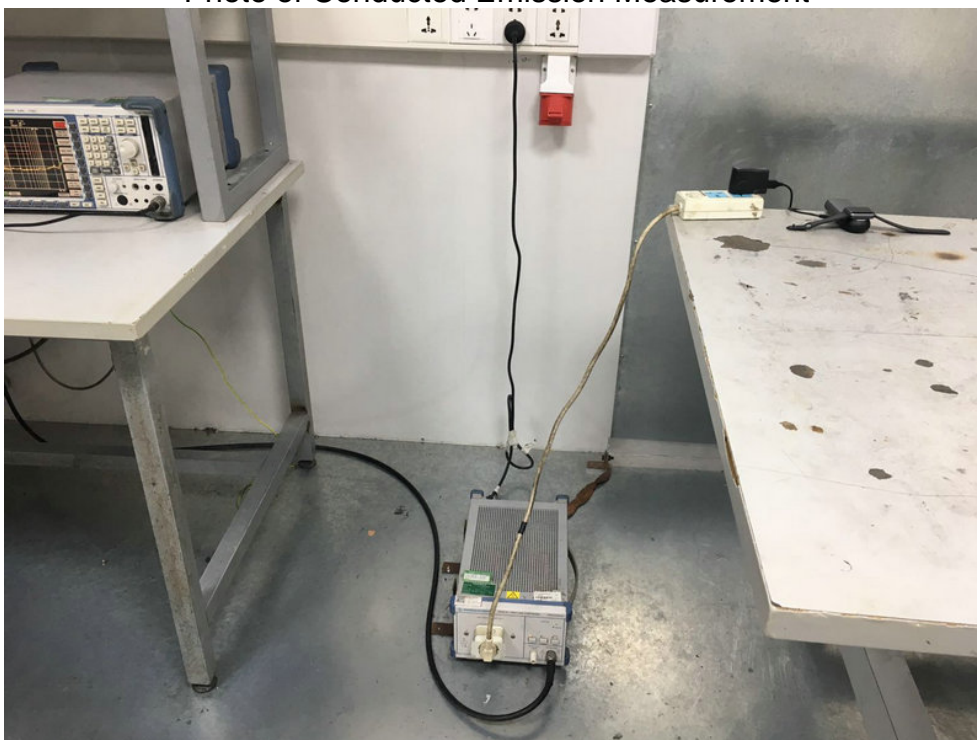
Photo of Conducted Emission Measurement
