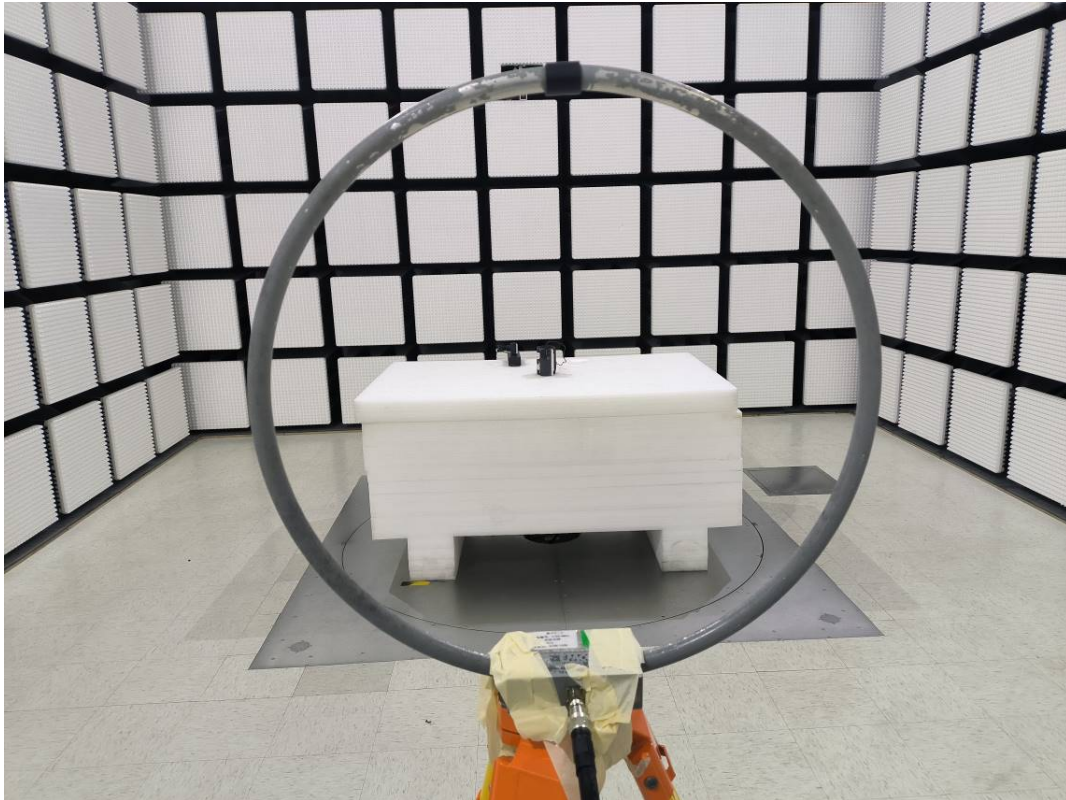
Radiated Emission 9kHz-30MHz Perpendicular View
