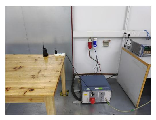
RADIATED EMISSION TEST SETUP-BELOW 1GHZ
