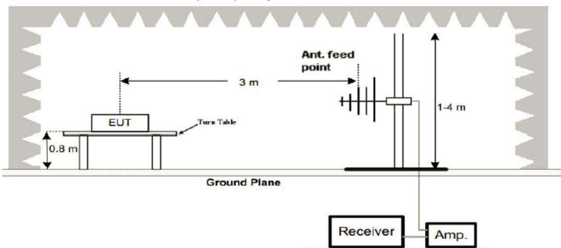
(3) Radiated Emission Test-Up Frequency Above 1GHz
