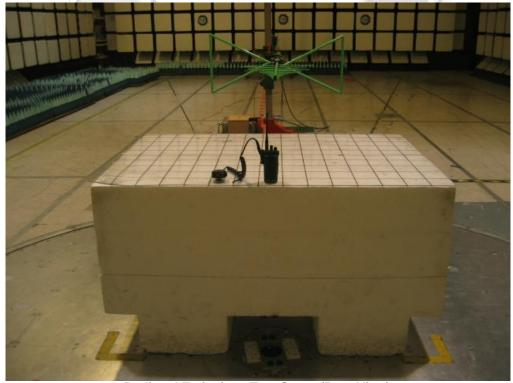
Radiated Emissions Test Setup (Rear View)
