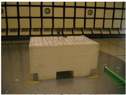
Radiated Emissions Test Setup (Front View)
