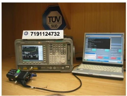
**Peak Power Spectral Density Test Setup**
