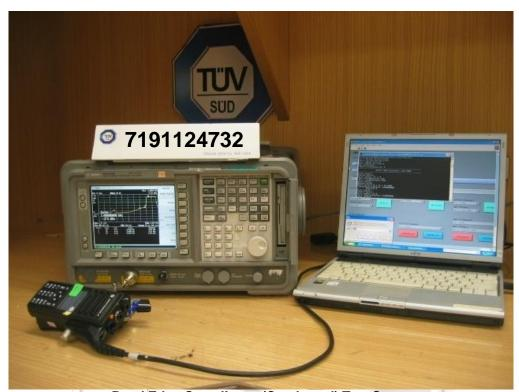
Band Edge Compliance (Conducted) Test Setup
