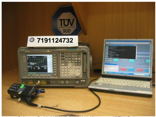
Spectrum Bandwidth (6dB Bandwidth Measurement) Test Setup
