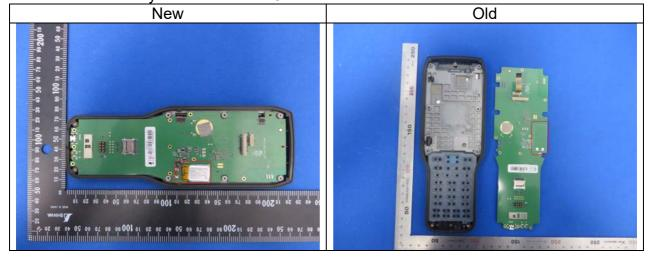
• Adding detachable batteries were added, one battery used LG Cell, another battery used Samsung cell.
