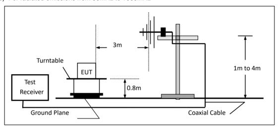
(c) For radiated emissions above 1000MHz
