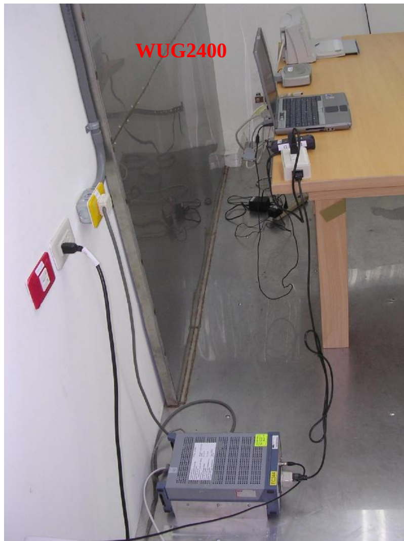
Photo 2: Conducted Emission Test Set-up
