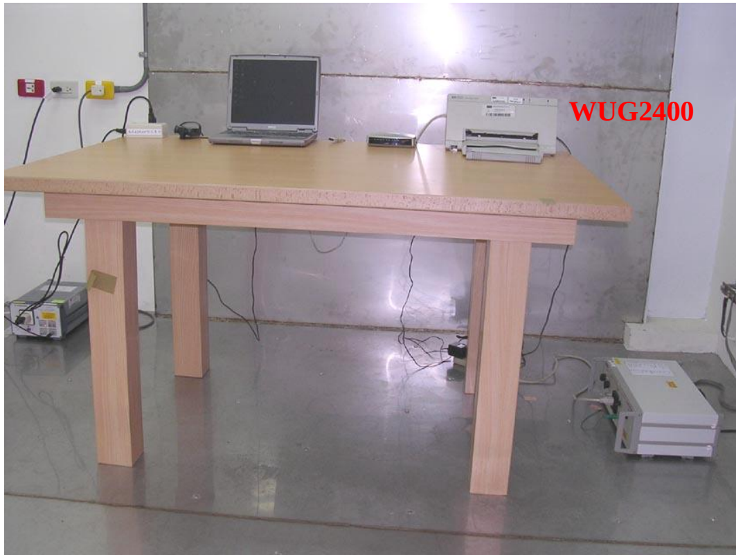
Photo 1: Conducted Emission Test Set-up
