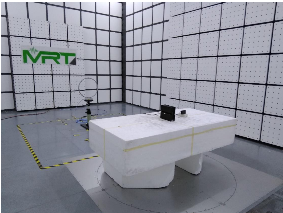
Description: Radiated Emission Test Setup for 9kHz~30MHz
