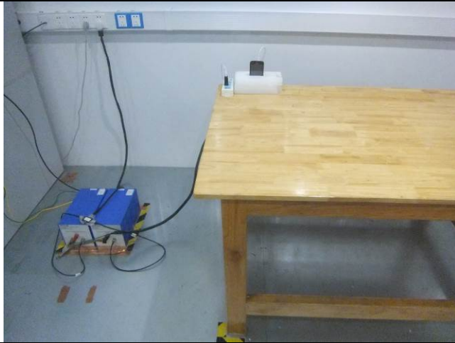
Conducted Emissions Test Setup Front View
