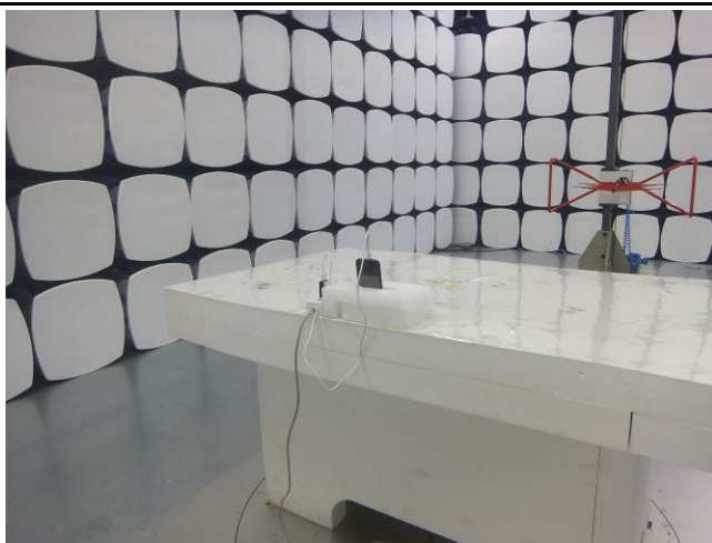
Conducted Emissions Test Setup Front View
