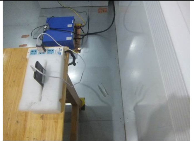
Conducted Emissions Test Setup Side View
